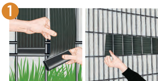
Waive the fence tape onto the panel.
