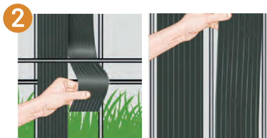
Fasten the tape in the end clip.
